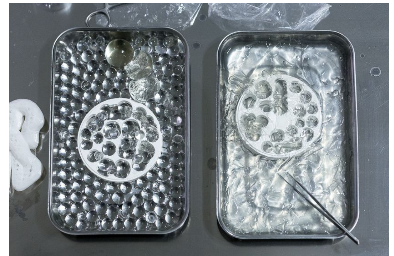
OP bowls with gel balls, gelatine and zirconium blanks from the dental laboratory
